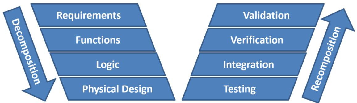
**Figure 9: Schematic Overview of the RFLP Process (Adapted from [46])**
