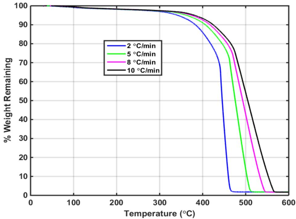
Figure 10. Sample Set of 4 Standard TGA Tests of KFA5 in zero-moisture Air at 2, 5, 8, and 10 °C/min
