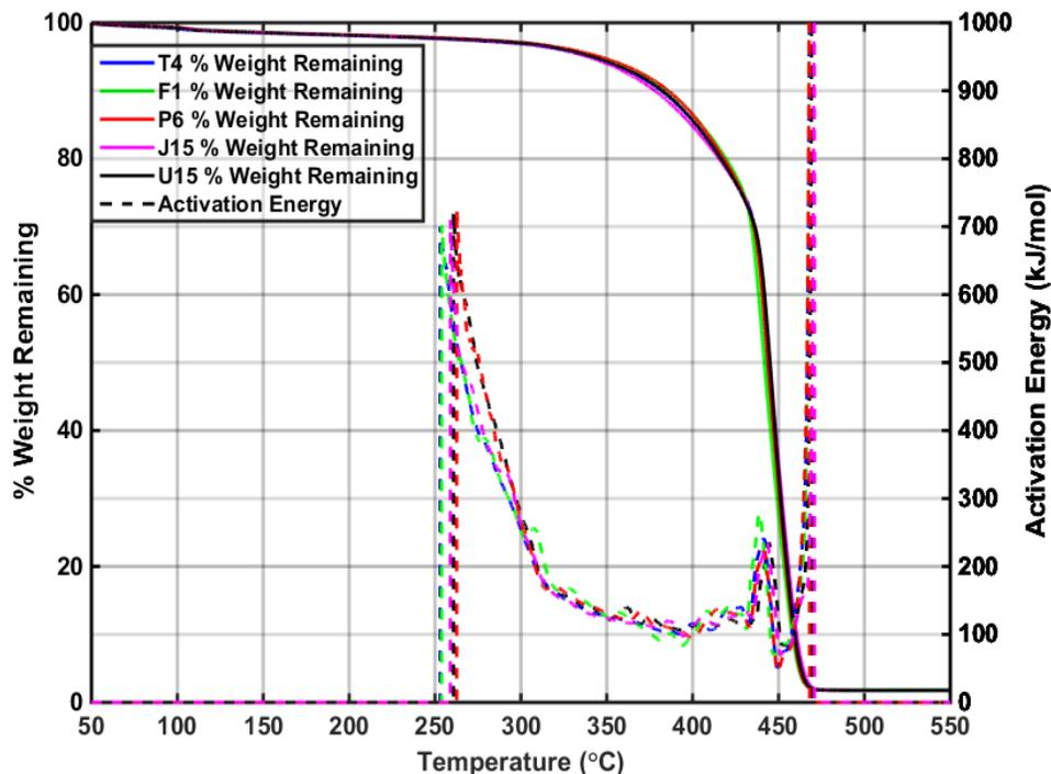
**Figure 12. 5 Sample Modulated TGA Tests of KFA5 in zero-moisture Air at 2 °C/min**
