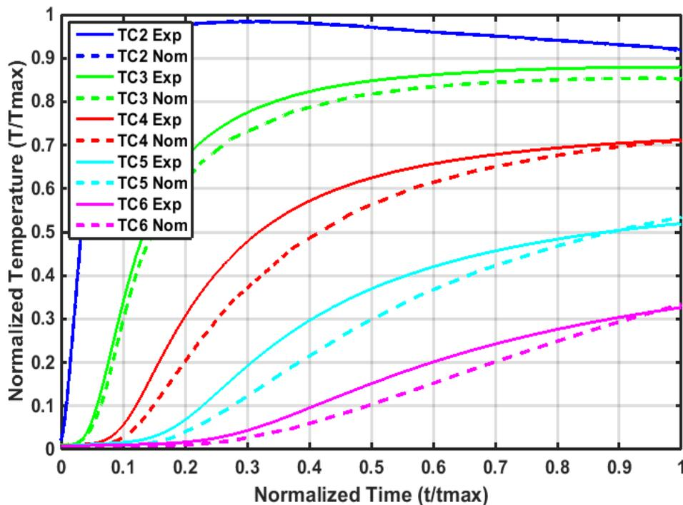
**Figure 15. Initial FTPS Thermal Response Model Comparison Between Normalized Arc-Jet Thermocouple Measurements at Depth (Lines) and Nominal Predictions (Dashes) for KFA5 Run 2659**
