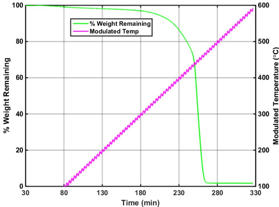
Figure 8. Sample Modulated TGA Test of KFA5 in zero-moisture Air at 2 °C/min
