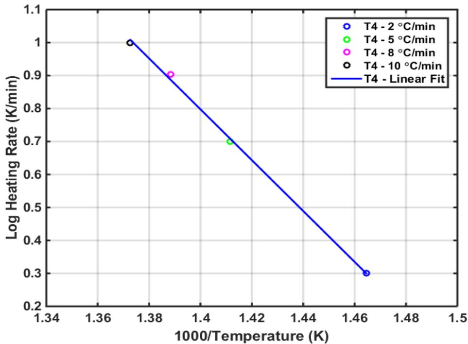
Figure 11. Sample Arrhenius Plot for a Set of 4 Standard TGA Tests of KFA5 in zero-moisture Air at 2, 5, 8, and 10 °C/min with a Linear Fit
