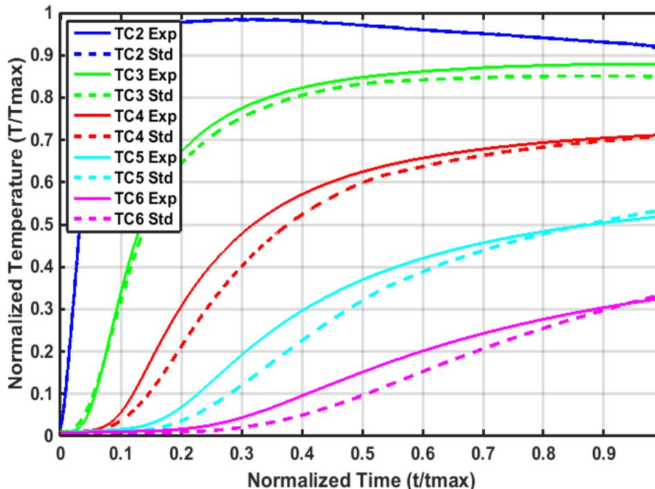
**Figure 16. Improved FTPS Thermal Response Model Comparison Between Normalized Arc-Jet Thermocouple Measurements at Depth (Lines) and Improved Predictions (Dashes) Using Activation Energy Determined from Standard TGA for KFA5 Run 2659**
