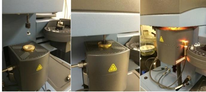
**Figure Set 4. Sample Loading Procedure of KFA5 Samples into TA Q5000IR**
