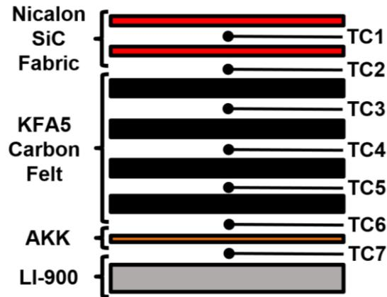
Figure 1. Pure KFA5 Layup (SiC, KFA5, AKK) <sup>4</sup>
