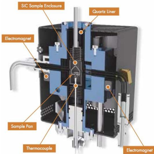
Figure 3. TA Q5000IR Furnace Cross Section <sup>15</sup>
